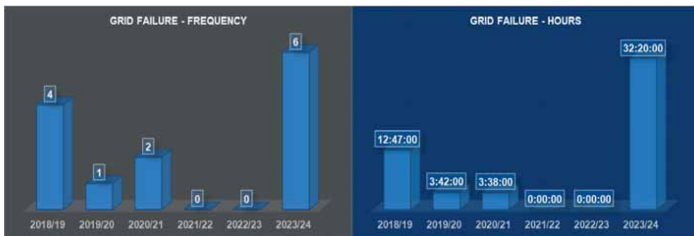
Figure 53: Total Grid Failure Frequency and Hours
