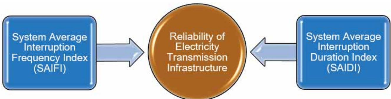
Figure 50: Description of Electricity Transmission Infrastructure Reliability Indices
